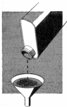
Always strain fuel when filling tank or priming engine. Strainer caps are available.
